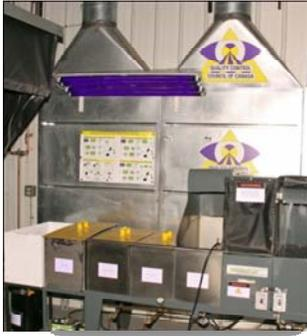
Figure 3 - Liquid Penetrate Station.
